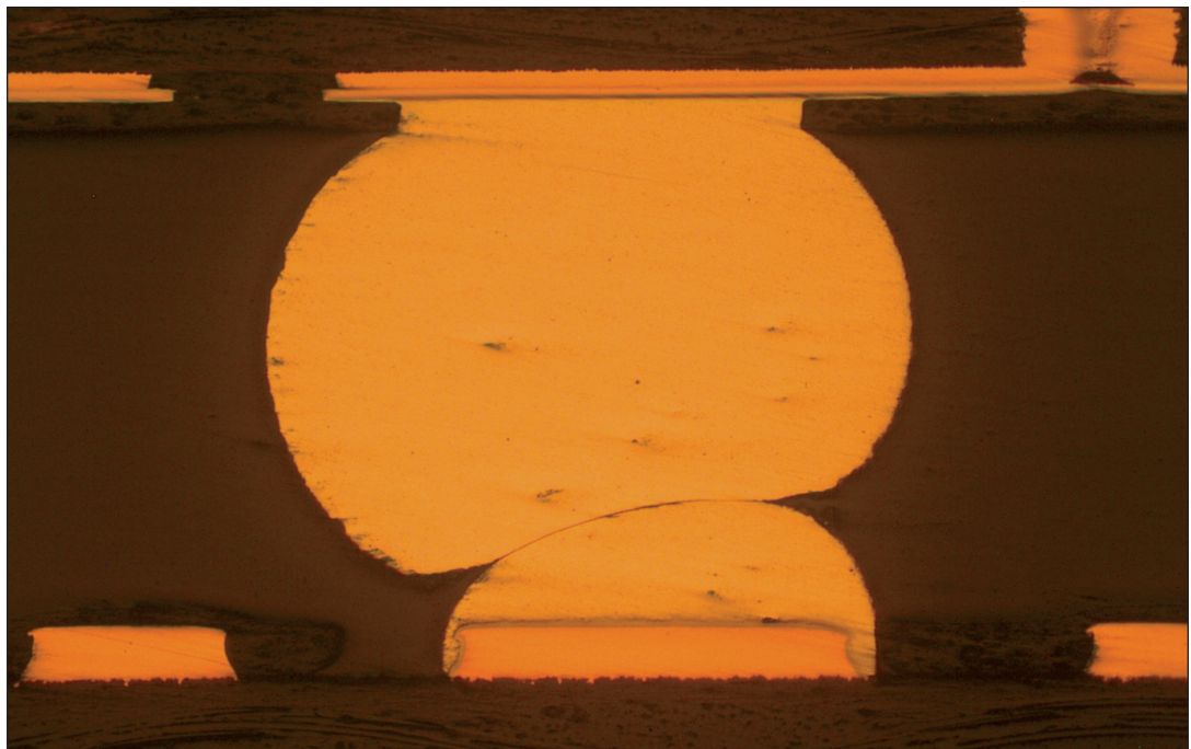
Figure 3-4: Metallographic image of a head-on-pillow defect on a BGA assembly.
