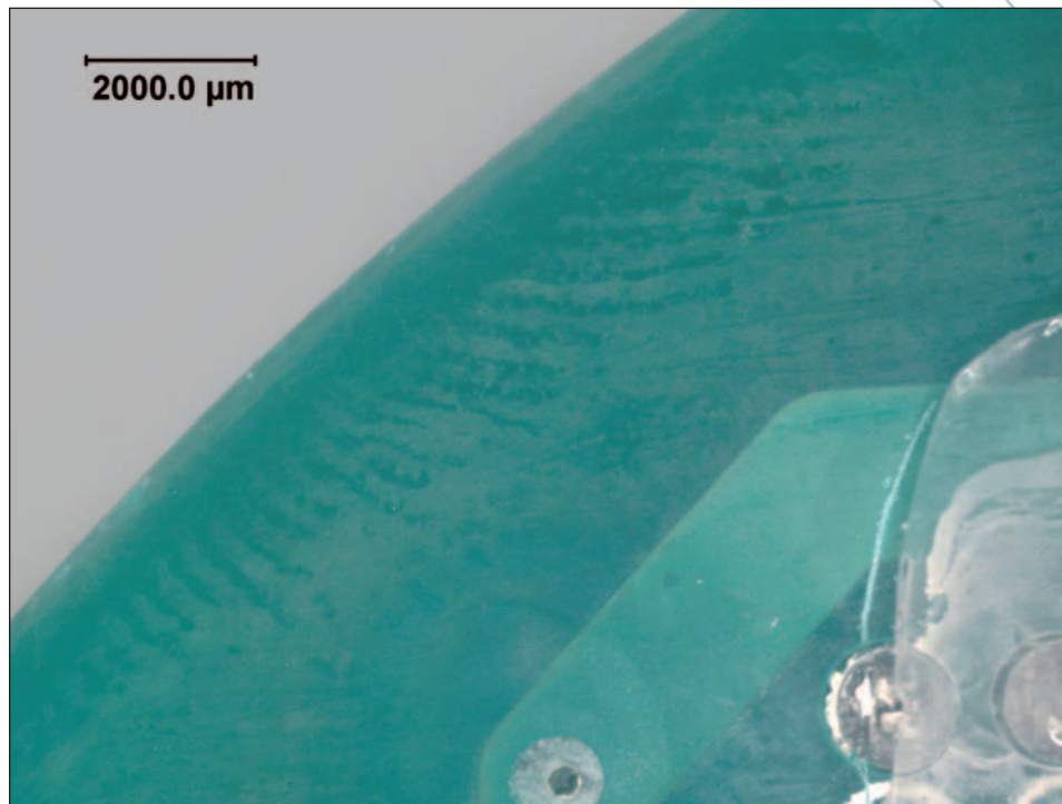
Figure 4-3: The oils from this fingerprint contributed to poor adhesion of the conformal coating and led to corrosion of unprotected metal surfaces.
